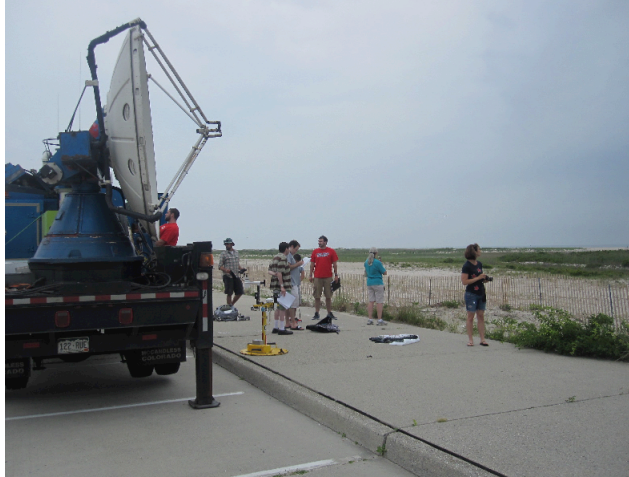
Figure 8. DOW deployment at Jones Beach on the Long Island south shore sampling convective storms over the Atlantic Ocean.
