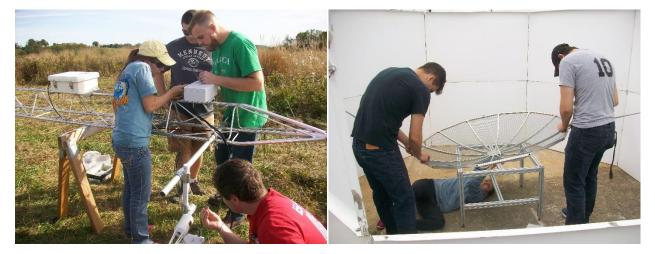
Figure 37: Students attach instruments to the 10 m flux tower (left) and anchor the RASS dish on the SoDAR (right). In addition, students were required to learn the theory of operation of all the sensors on each platform.
