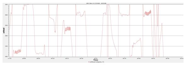
*Figure 30: King Air aircraft true aircraft heading measurements. Note the three periods of regular variation that represent a series of maneuvers to vary yaw via the rudder.*
