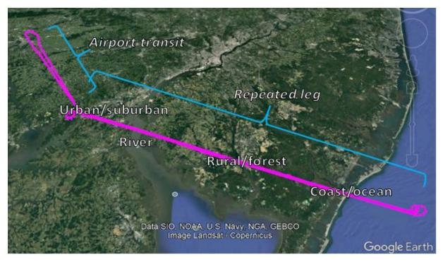
Figure 20: Flight track for the RF09 PBL Height Variation science mission on the afternoon of 11 NOV 2017. The PBL in the mid-Atlantic region is uniquely complicated by the convolutions created by land, rivers, large bays, and ocean. The repeated leg was flown four times between Elkton, MD on the west end and 10 miles off the NJ coast on the east end.
