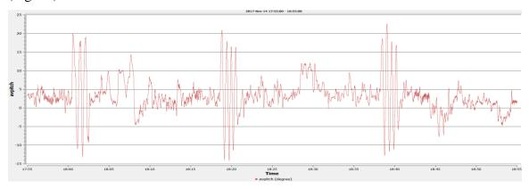
Figure 34: King Air aircraft pitch measurements. Note the three periods of regular variation that represent a series of porpoising maneuvers.
