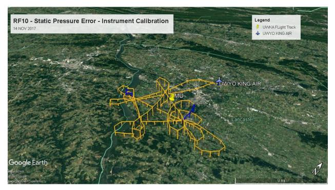
Figure 31: Flight pattern used for the determination of the aircraft static pressure error. The pattern was designed to maximize the variation in aircraft parameters (pitch, roll, yaw, airspeed, etc.) and to gather a sufficiently long data set to provide a statistically robust algorithm with which to estimate the error in static pressure measured at the static ports.
