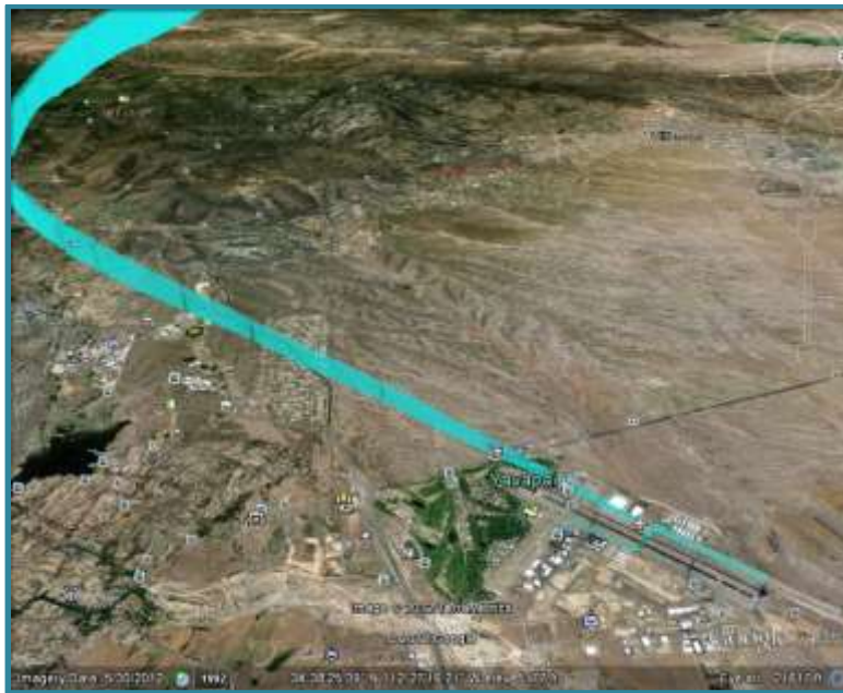
Fig. 2. Example of approach and landing at KPRC airfield by an ERAU pilot training flight. The primary runway is oriented at 030-210 deg. The approach trajectory indicates higher terrain to the west of Prescott associated with the Granite Mountain range.
