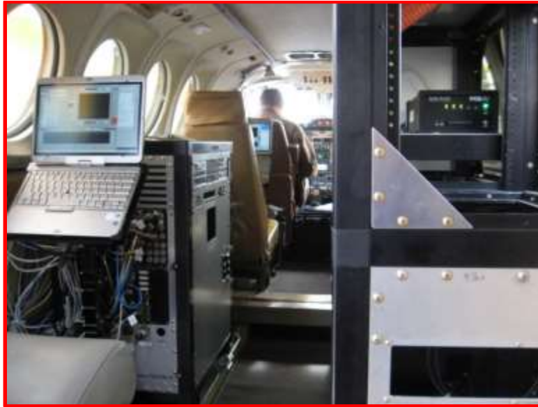
Fig. 5. Interior view of UWKA from entryway, showing instrument racks, data access / visualization computers used by onboard scientists (ERAU students and faculty), and pilot Tom Drew. Additional seats are located on the right side of the aircraft -- in the cockpit next to the pilot (allocated for ERAU faculty) and immediately to right of the middle console (allocated for UW lead scientist). Each of these seats also have data visualization computer systems.
