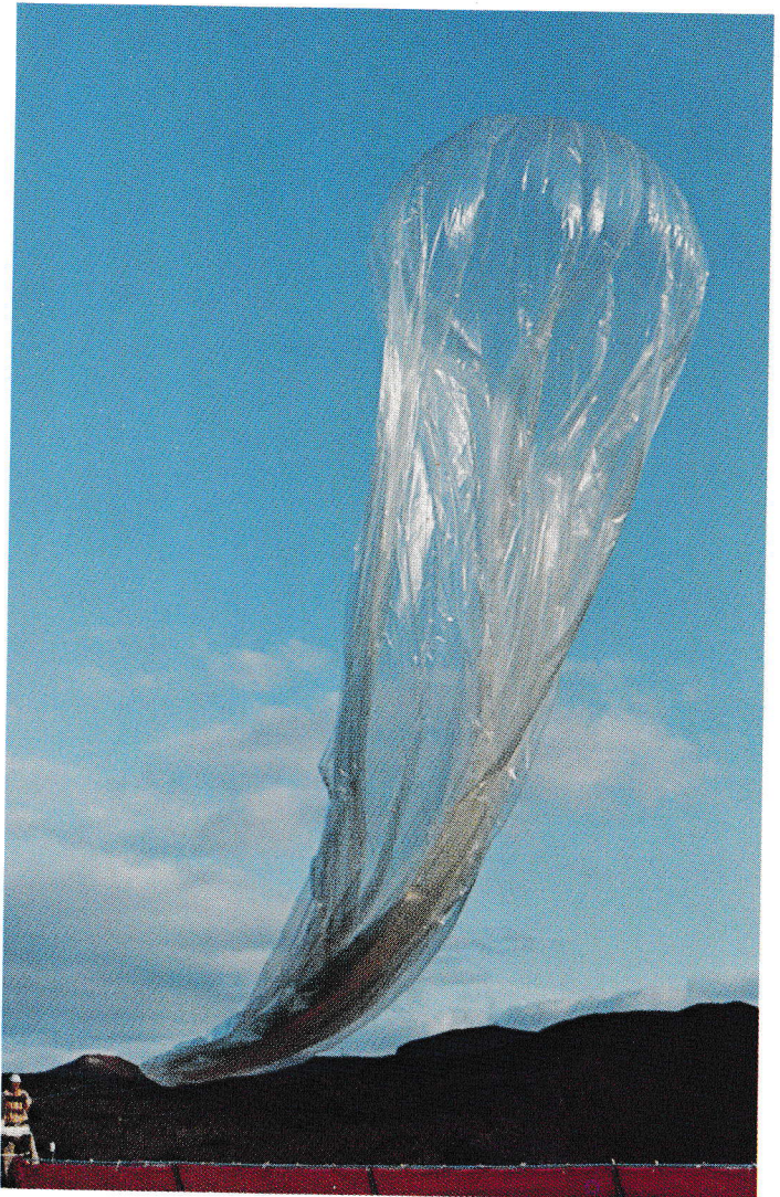
The large size (12 m diameter) of 30 mb balloons and the strong trade winds at Ascension Island necessitate special launching techniques. The partially inflated balloon is held under a nylon cover in a "GHOST wagon" while a towing vehicle drives downwind to neutralize the wind speed. The cover is then opened, allowing the balloon to rise undisturbed.
