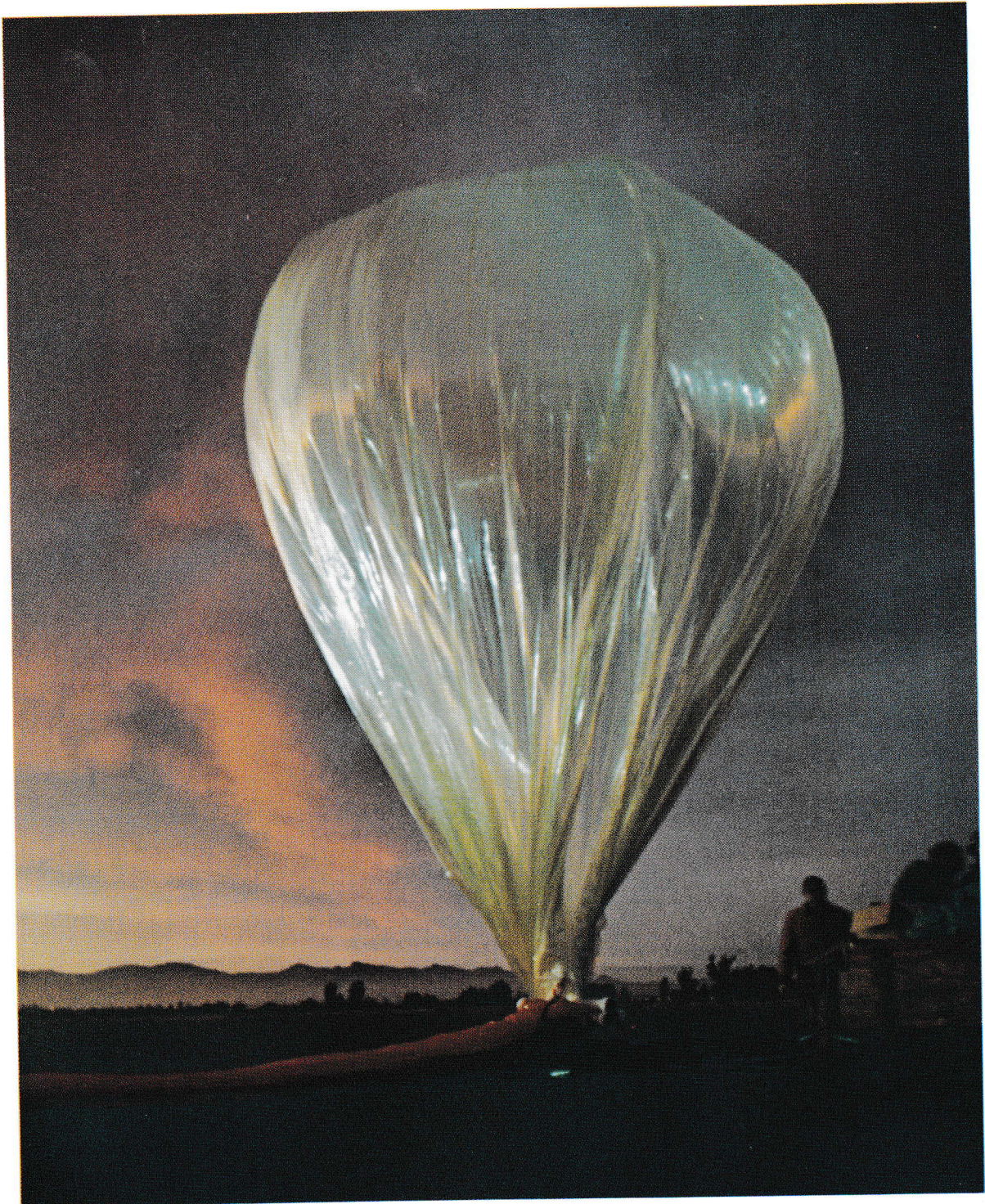
The Carrier Balloon/Omegasonde System (CBS) was designed to provide upper air data in areas where they are not available by other means. The CBS involved large (21.4 m diameter) superpressure balloons carrying cargoes of miniature dropsondes. The sondes were released on radio command and their reports relayed by the carrier balloon to a satellite and then to earth. This system was developed by NCAR to provide a means of obtaining wind profiles in equatorial regions to meet the goals of the Global Weather Experiment. Field tests of the complete system were completed at Kourou, French Guiana.
