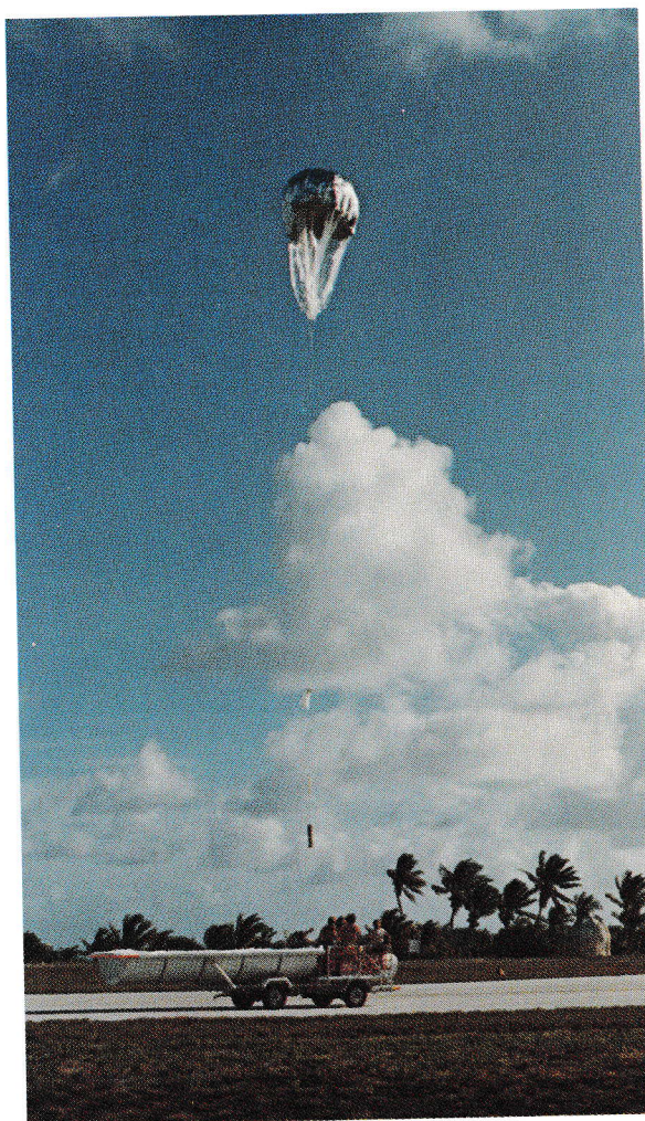
The mobile launch technique, adopted from the TWERLE program, easily allowed launching of 313 TCLBS platforms from Ascension Island (South Atlantic), Canton Island (central Pacific), and Guam (western Pacific). At the time of launch, the balloon is only partially inflated to allow for expansion of the helium as the balloon rises and the atmospheric pressure decreases. When the mass of air displaced equals the mass of the balloon plus its payload, the balloon stops rising and floats at this density level, moving with the air circulation.
