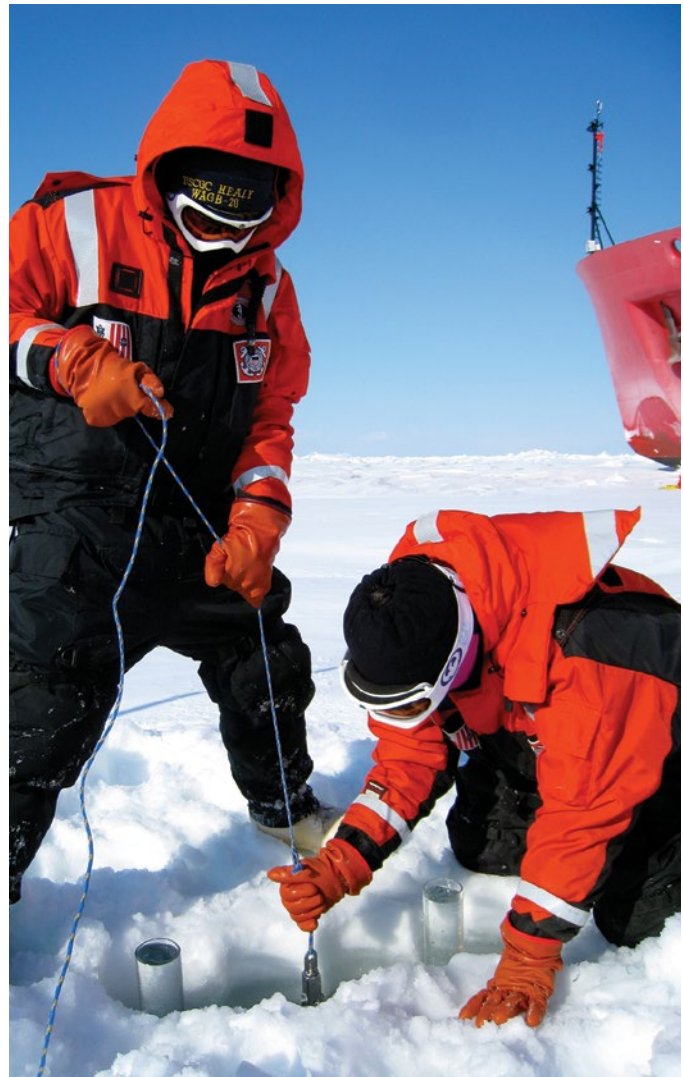
Deploying a "sediment trap" to measure the 'export' or sinking of ice algae from the ice to the seafloor.
