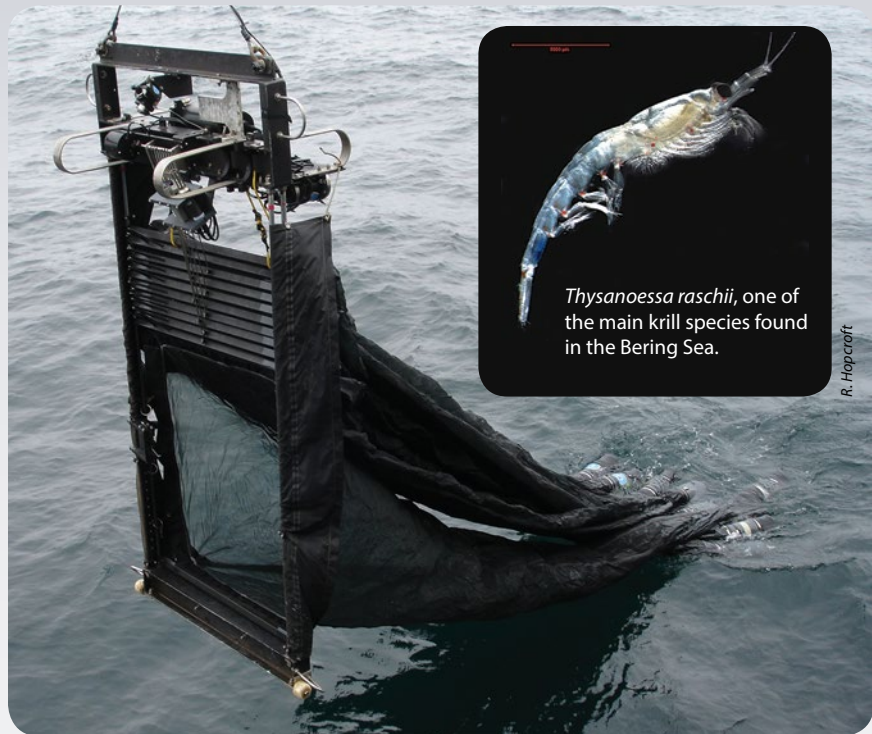
Deployment of a “multiple opening and closing net with an environmental sensing system”, aka “MOCNESS”—this specialized net can collect krill samples at different depths during a single tow. The frame carries 9 separate nets.
