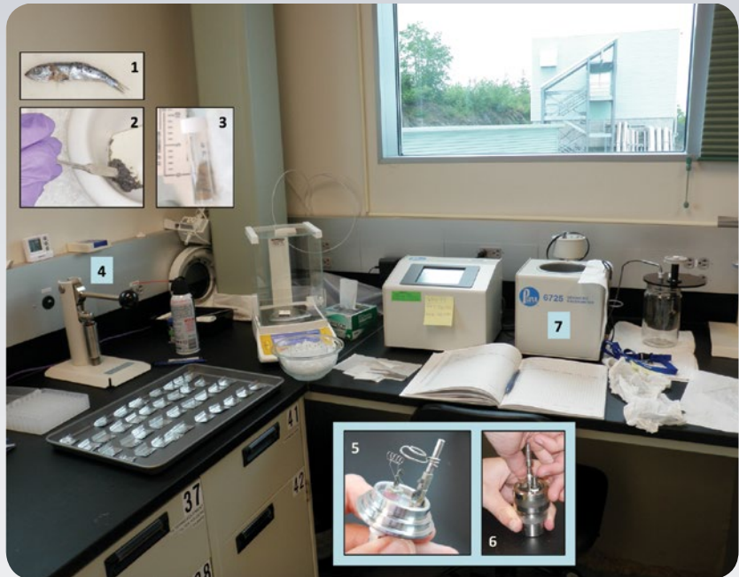
A bomb calorimetry setup, showing all the various components. Fish (1) are ground up (2) and dried into a powder (3). A sample of the powder is pressed into a pellet (4) and loaded into the pellet holder (5), which has a fuse installed. The pellet and fuse are loaded into the bomb casing (6) and the casing is filled with oxygen and then placed in the water bath (7). Electrodes heat the fuse, which ignites the powder and the heat warms the water bath. A thermometer in the water bath records the change in temperature. The computer converts the temperature change into calories. One calorie is the amount of heat necessary to warm one cubic centimeter of water 1°C.
