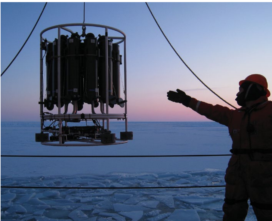
US Coast Guard marine science technicians aboard the icebreaker USCGC Healy deploy the Niskin rosette water sampler together with the CTD (conductivity-temperature-depth). This package of instruments retrieves water samples from specific depths, and creates a ‘profile’ of the salinity and temperature along the entire water column. After being brought back aboard, the Niskin water sampling bottles are the hub of intense activity as multiple research teams extract samples from the bottles.
