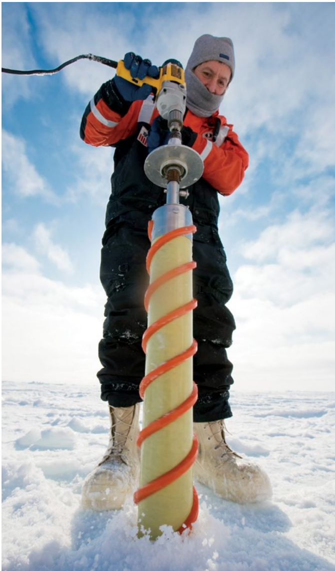
Project scientist Rolf Gradinger taking ice samples with an ice corer.
