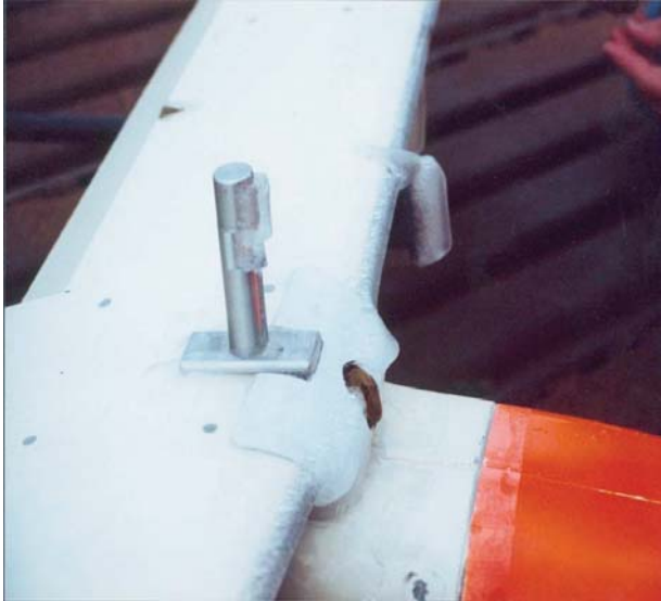
FIG. 1. Ice on the leading edge of an Aerosonde together with an early icing device (the vertical tube) and the current piezoelectric device mounted on the leading edge of the wing (the device inside the circular opening above the fuselage).
