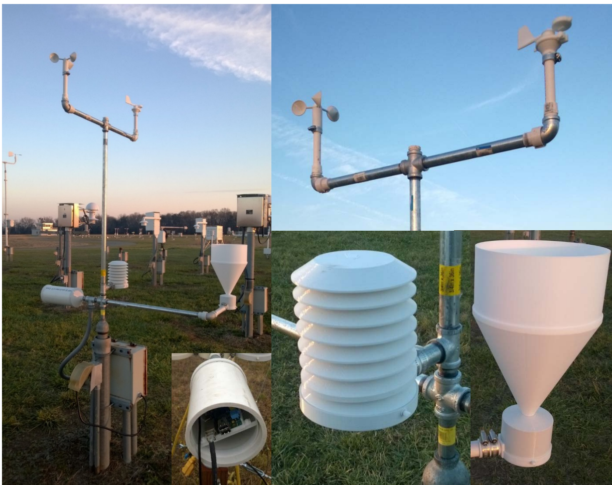
Figure C1. Photos of a 3D-PAWS setup. The left images shows the complete setup. The upper-right photos shows a close up view of the 3-cup anemometer (left) and wind vane (right). The bottom photos show images of the Raspberry Pi housing, radiation shield, and tipping bucket rain gauge.
