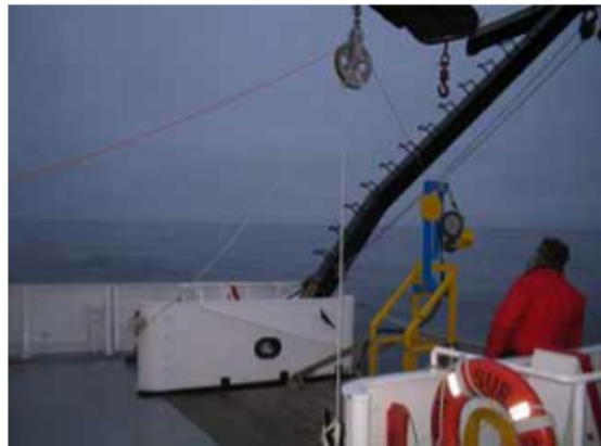
Figure 5: VMP winch system setup, with the spool unit (left) about 20 ft forward of the line-puller unit (right), which is directly on the stern under the A-frame. A Sherman-Riley block is suspended just fore of the line puller (this arrangement can be done by tilting the A-frame forward).
