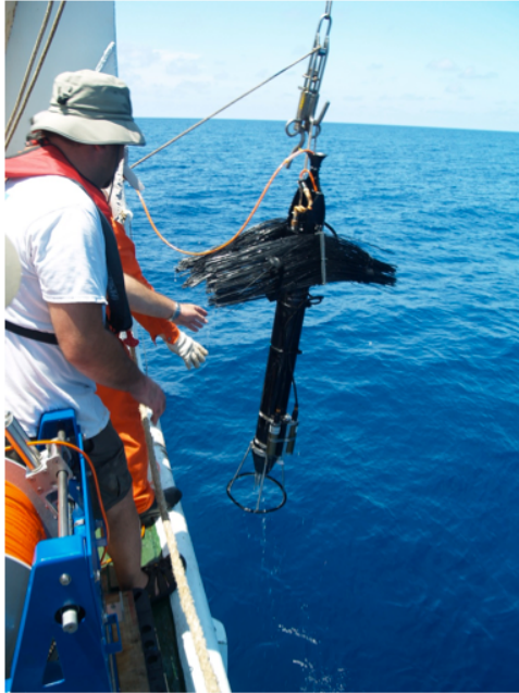
Figure 4: The 500-m rated Rockland Scientific Vertical Microstructure Profiler (VMP-500). The sensors are located at the nose, protected by a guard ring. Drag whiskers are deployed at the tail. The tether terminates through a strain relieve component.
