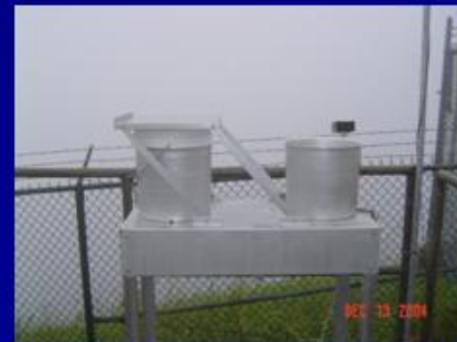
Rain water collector
