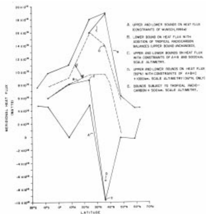
Figure 2. Meridional heat flux bounds on the Atlantic circulation under various assumptions. The outermost curves are the maximum and minimum from paper A. At low latitudes, the minimum is strongly affected by the demand for consistency with C-14 constraints of paper B. At mid- and higher latitudes, simulated sea level constraints make a significant impact on the bounds.
