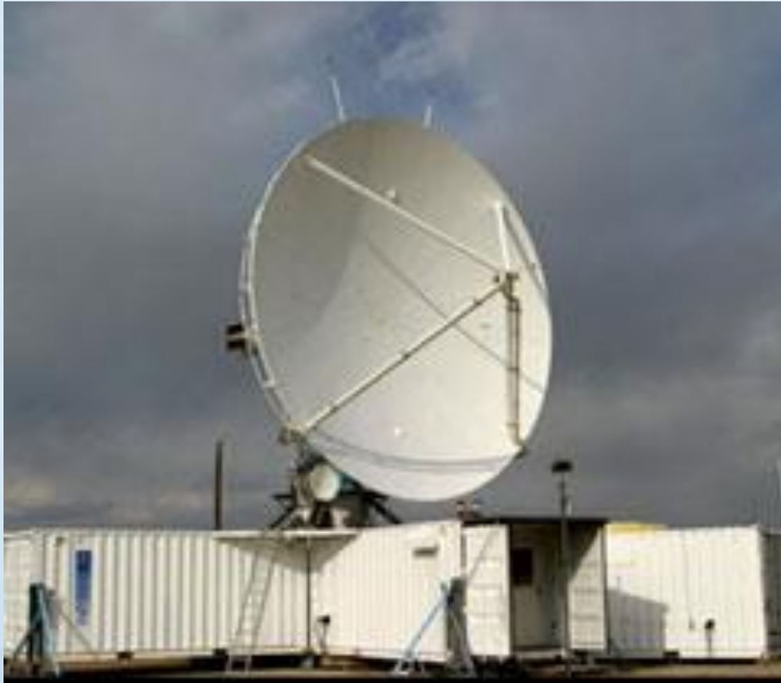
S-Polka radar system at the Marshall field site near Boulder during WISP04 project.
